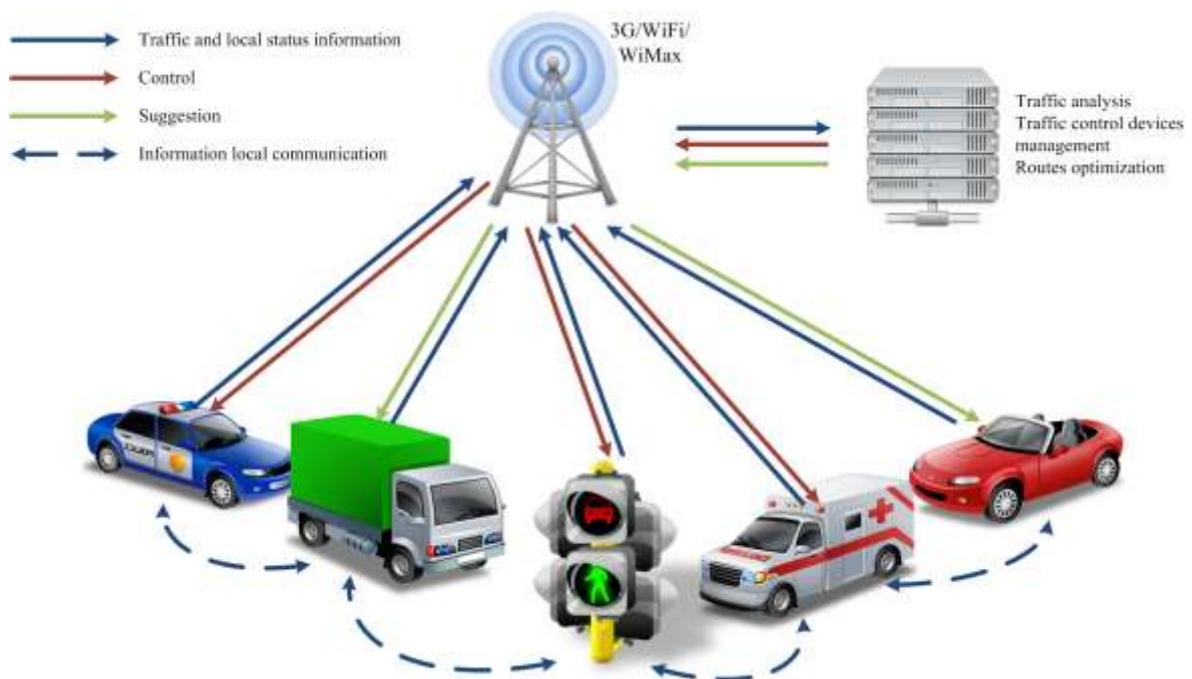
Vehicles send local information to a central server that uses it to manage the traffic, to plan best routes for emergency vehicles and optimize traffic lights behavior. Local communication between vehicles can be used entertainment and safety (e.g.: collision alarm).
